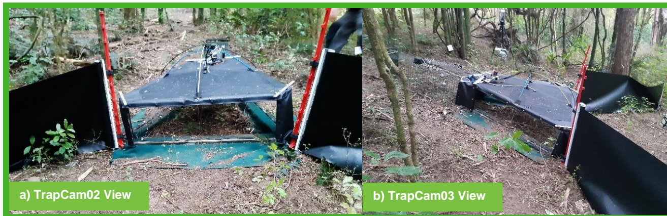
Figure 5. Photographs of the Cacophony prototype trap at the first field-test location at Living Springs (43°39'19.4"S 172°37'53.4E): a) Front view, b) Side View. Additionally, these photos align with the view of the Cacophony thermal cameras used to monitor the trap: a) TrapCam02, b) TrapCam03 (© Saphy Hampshire).
