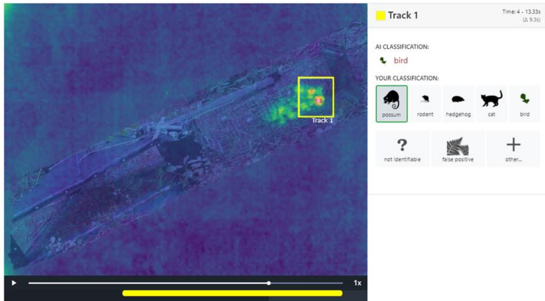
Figure 10. Example of footage from TrapCam01 (Cacophony thermal camera) monitoring the Cacophony prototype trap (Side View). The recording shows a possum trapped in the back cage of the trap and an overlay has been added to highlight the trap outline on the recording (© The Cacophony Project).
